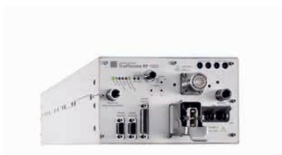
Extremely robust RF generator for PECVD and etching applications in semiconductor manufacturing. Accurate output power regulation and CombineLine allow for stable processes and best productivity. Cost-efficient system integration due to compact half 19" design.
