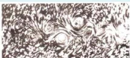
Vertex street observed downstream of a bluff delta-shaped object with sharp edge
